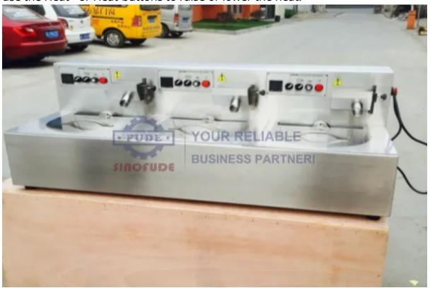
The chocolate should flow into a cooling zone at the correct temperature. The temperature is usually displayed on the control panel. Make sure that the temperature of the chocolate is not too hot or too the temperature is too high, it will lead to sugar blooming. To avoid this, you must make sure that the humidity in the cooling section is between 63 and 70%. If the chocolate is too warm or too cool, it makes the cooling process.
