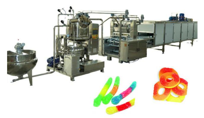
The first step in using a gummy machine is to gather ingredients. The ingredients are placed in the hore The gelatin is heated to a liquid state. This allows the mixture to flow freely and gives it the desired sh hopper is also filled with predetermined sizes of the candy. The machine's design includes a metal vib sequence that helps to distribute the gelatin evenly throughout the entire hopper.
